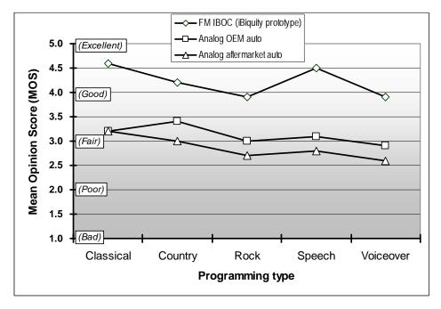
Figure 7. Comparison of FM IBOC and analog audio subjective evaluation results aggregating all field test conditions<sup>17</sup>
