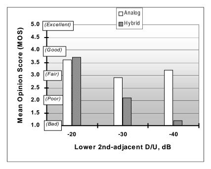
Figure 21. 2nd-adjacent compatibility – subjective test results with analog and hybrid interferers (home hi-fi receiver, lower 2nd-adj., with 30,000K noise)
