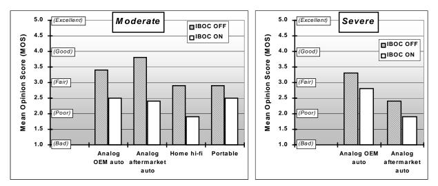
Figure 10. 1st-adjacent compatibility - subjective evaluation results of audio recordings obtained in the field (speech programming) Moderate: +16 to +6 dB D/U Severe: +6 to -9 dB D/U
