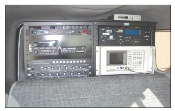
Figure 6. iBiquity prototype receiver –as used in field test vehicle (receiver is rectangular black box in upper right-hand corner of rack)
