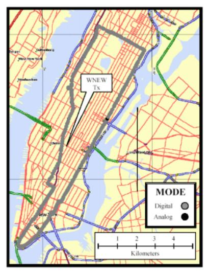
Figure 15. Map showing FM IBOC digital coverage along route in Manhattan, NYC.
