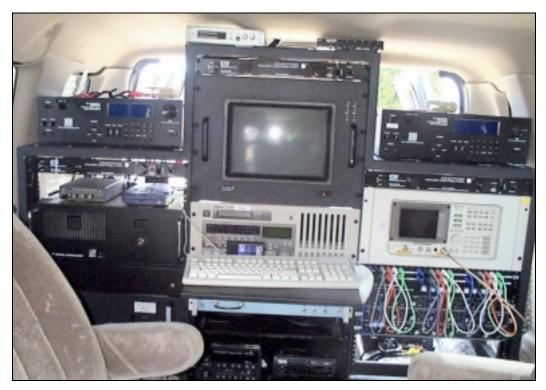
Figure 5. Interior view of field test vehicle showing analog and IBOC receivers, computer, and test equipment
