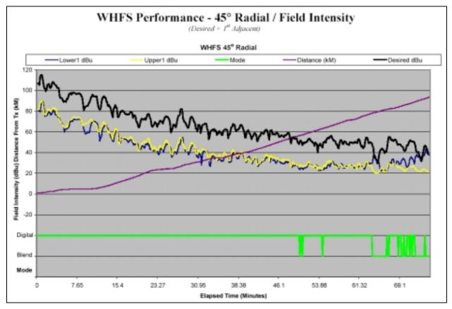
Figure 17. Field test signal strength graph (WHFS, 45° radial)
