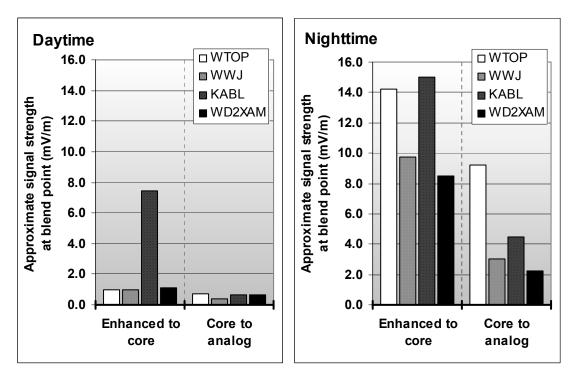
Figure 23. Approximate signal strength at blend points for field test stations (for each station, results averaged over all test radials)
