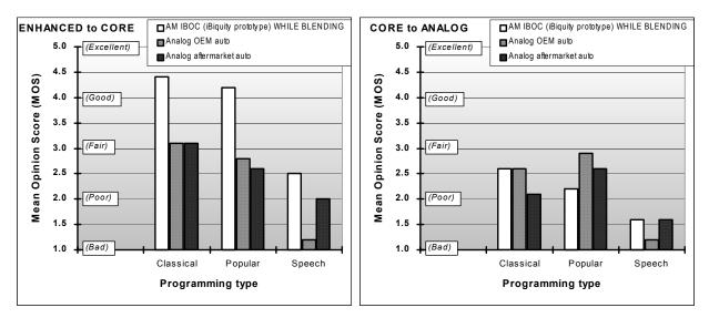
Figure 26. Comparison of AM IBOC and analog audio subjective evaluation field results at "blend to analog" operating point
