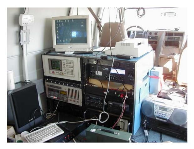
Figure 6. Interior view of field test vehicle showing analog and IBOC receivers, computer, and test equipment
