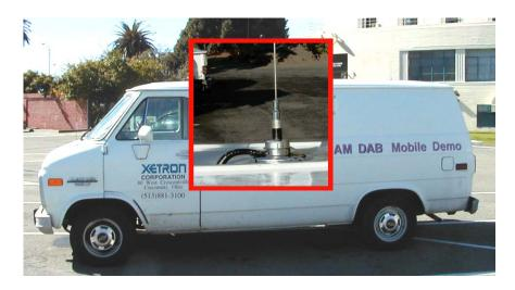
Figure 5. Field test vehicle and roof-mounted receive antenna (inset)
