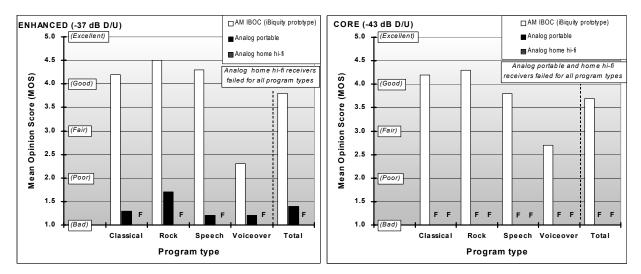
Figure 19. Comparison of AM IBOC and analog audio subjective evaluation results obtained in the laboratory with single 3rd-adjacent channel interference
