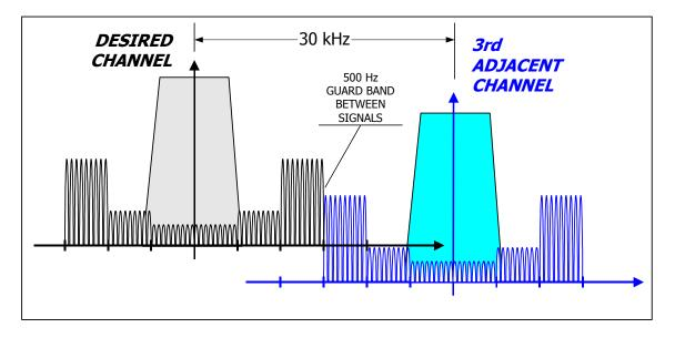
Figure 4. Illustration of potential interference between 3<sup>rd</sup>-adjacent AM IBOC signals
