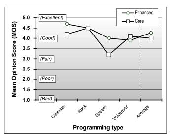
Figure 10. Comparison of AM IBOC subjective evaluation results for enhanced digital and core digital audio quality under laboratory AWGN conditions
