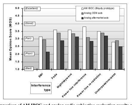
Figure 20. Comparison of AM IBOC and analog audio subjective evaluation results obtained in the field in the presence of various forms of interference
