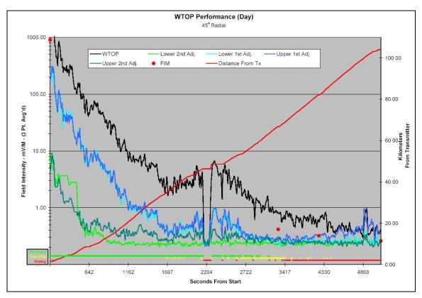
Figure 21. Field test signal strength graph, daytime (WTOP, 45° radial)
