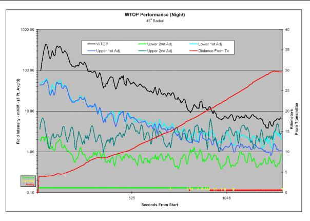
Figure 22. Field test signal strength graph, nighttime (WTOP, 45° radial)
