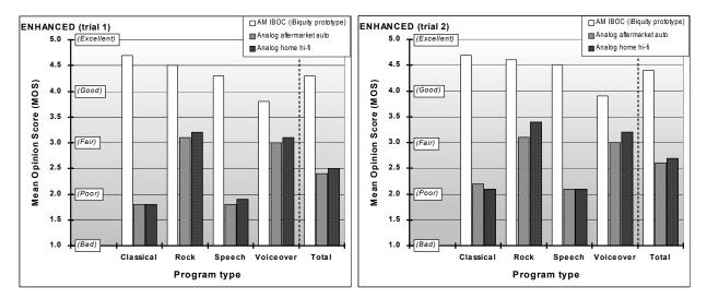
Figure 13. Comparison of AM IBOC and analog audio subjective evaluation results obtained in the laboratory with co-channel interference (+17 dB D/U)
