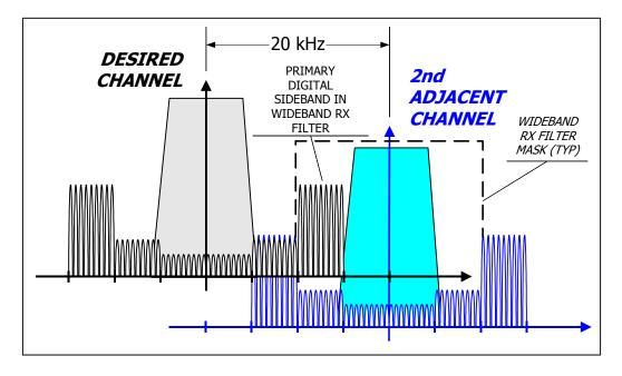
Figure 3. Illustration of potential interference between 2<sup>nd</sup>-adjacent AM IBOC signals
