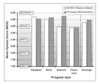
Figure 11. Comparison of AM IBOC and FM analog subjective evaluation results aggregating all laboratory test conditions<sup>24</sup>
