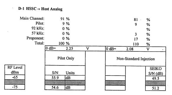
Measurements made Q-Peak detected with CCIR weighting and 15 kHz low pass filters (psophometric).
