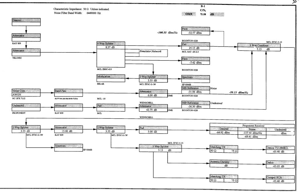
B-1 Additive White Gaussian Noise Characterization of HS Digital Subcarrier Signal Failure
