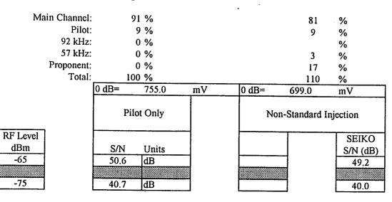
Measurements made Q-Peak detected with CCIR weighting filter (psophometric). 0 dB Reference Measurements made with 1 kHz Mod Source on Main Channel L+R. Measurements on Left Channel
