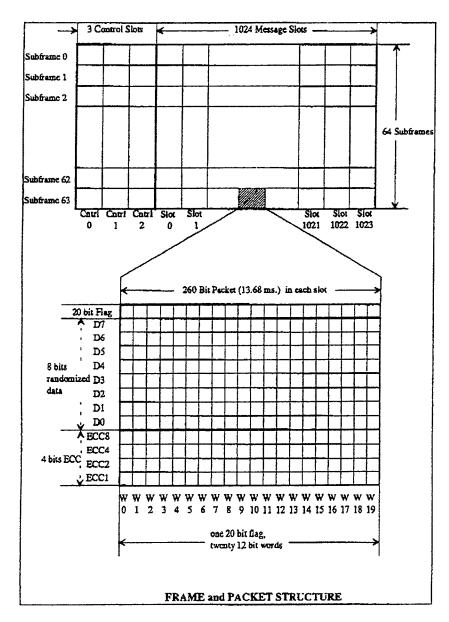
Figure 2 Frame and Packet Structure
