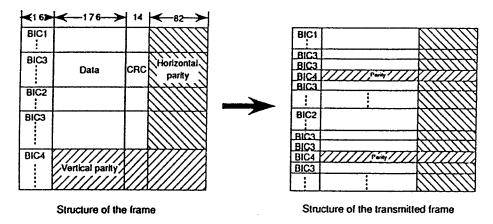
Figure 3. Structure of the frame
