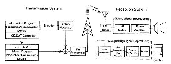
Figure 2. FM multiplex broadcasting system (Parts of slant lines are that we developed recently)
