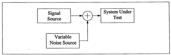
Figure 1. Approach used in HSSC Tests to Vary Signal-to-Noise Ratio
