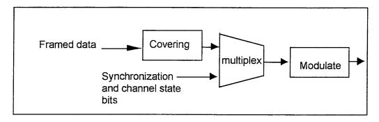
Figure 2. Modulation Signal Processing Overview
