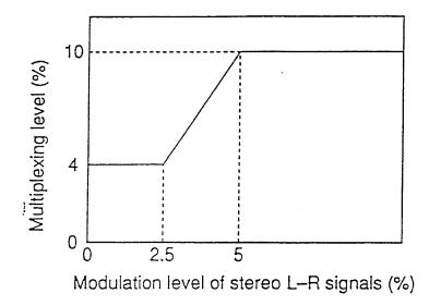
Figure 3. L-MSK method level control characteristics.
