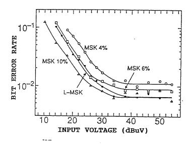
Figure 7, Input voltage vs. Bit error rate
