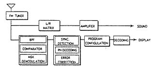
Figure 4. Block diagram of receiver
