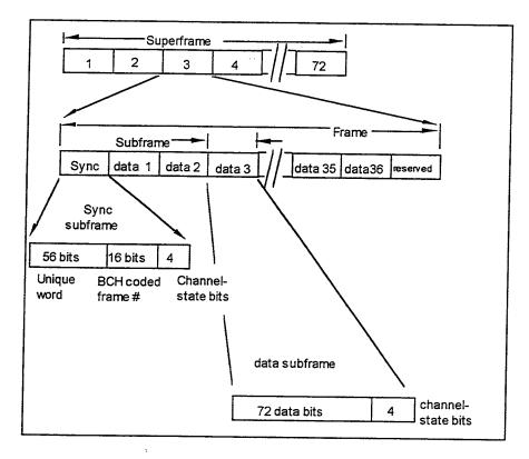
Figure 3. Example Frame Structure
