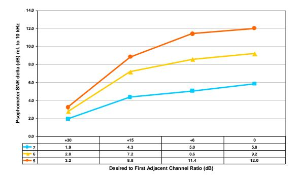
Figure 8. Effect of transmission bandwidth on received SNR
