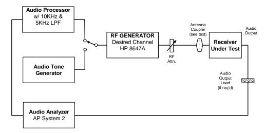
Figure 16 - Test Bed setup for audio performance measurements
