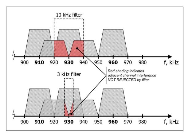
Figure 6. Illustration of the rejection of adjacent channel interference as a function of receiver filter bandwidth.
