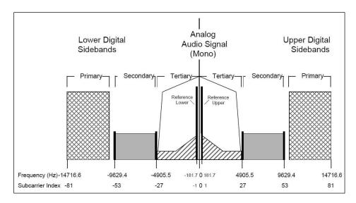
Figure 10. Hybrid AM IBOC spectrum - 5 kHz analog signal bandwidth8
