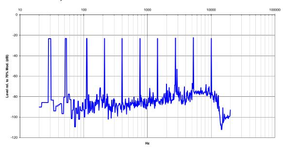
Figure M-4 - Spectral output mask of Optimod 9200 using USASI noise at lowpass filter bandwidths from 4.5 kHz to 9.0 kHz in 500 Hz increments.
