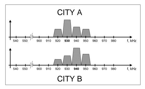
Figure 5. Elimination of first adjacent channel energy overlap in skywave reception conditions – ±5 kHz signals, nighttime
