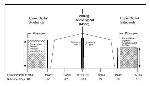
Figure 12. Hybrid AM IBOC spectrum – reduced digital bandwidth configuration<sup>10</sup>
