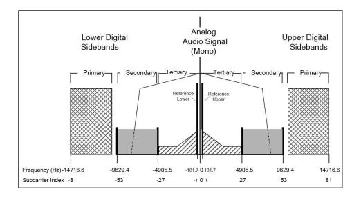
Figure 11. Hybrid AM IBOC spectrum - 8 kHz analog signal bandwidth9
