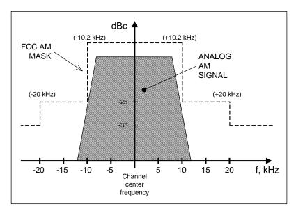
Figure 1. FCC analog AM mask
