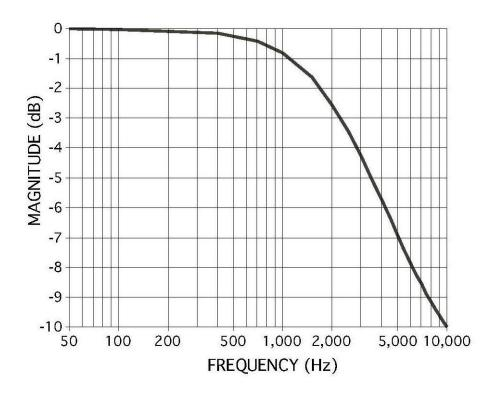
Figure 2. Modified 75µs AM Standard Deemphasis Curve
