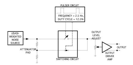
Figure 6. Pulsed-USASI Noise Generator
