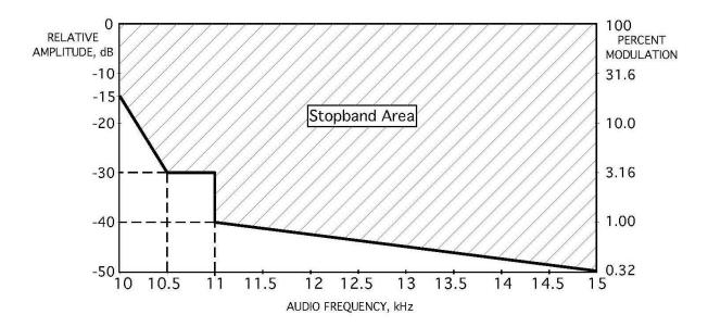
Figure 4. NRSC Stopband Specification for Analog AM Transmission
