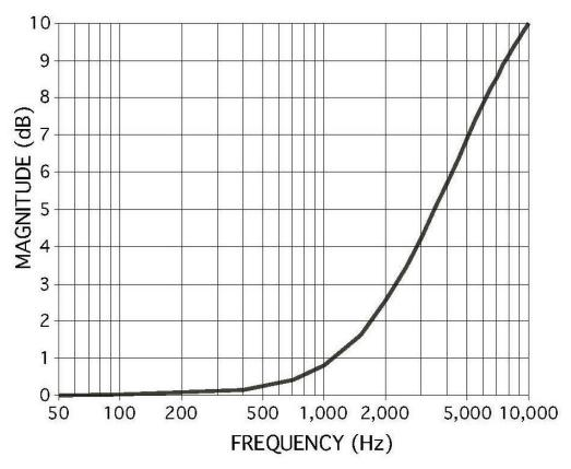
Figure 1. Modified 75 µs AM Standard Preemphasis Curve
