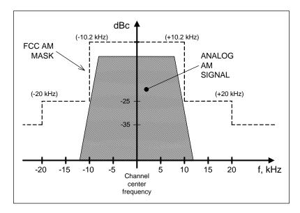
Figure 1. FCC analog AM mask
