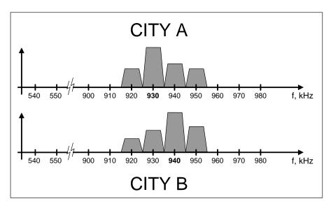
Figure 5. Elimination of first adjacent channel energy overlap in skywave reception conditions –  $\pm 5$  kHz signals, nighttime
