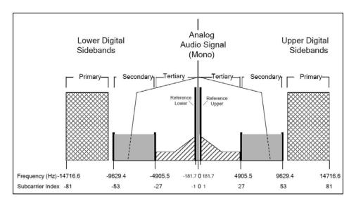
Figure 11. Hybrid AM IBOC spectrum – 8 kHz analog signal bandwidth<sup>9</sup>
