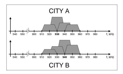
Figure 4. Illustration of interference from adjacent channel overlap of skywave signals from multiple stations – ±10 kHz signals, nighttime
