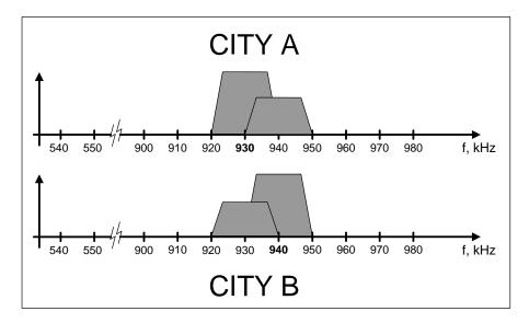
Figure 3. Illustration of interference from adjacent channel overlap of skywave signal – ±10 kHz signals, nighttime
