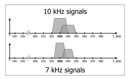
Figure 12. Illustration of reduction in first-adjacent channel interference when reducing signal bandwidth from 10 kHz to 7 kHz – the region of overlapped spectra represents the amount of adjacent channel interference in each case
