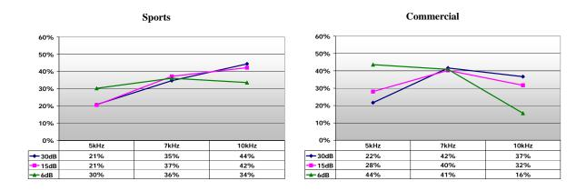
Figure 9. Percentages of listeners who picked one bandwidth over another, by genre, with no 1st-adjacent channel interference (30 dB), moderate 1st-adjacent channel interference (15 dB), and heavy 1st-adjacent channel interference (6 dB)
