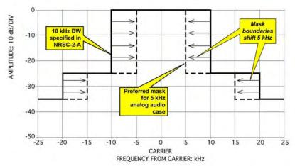
Figure 13. Illustration of preferred reduction of RF mask for example in Section 4.3
