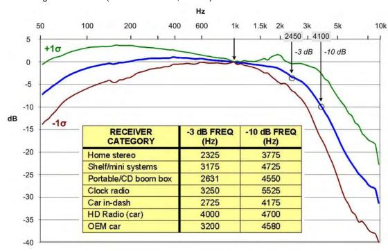
Figure 7. AM frequency response mean and standard deviation (1σ) curves for all measured receivers
