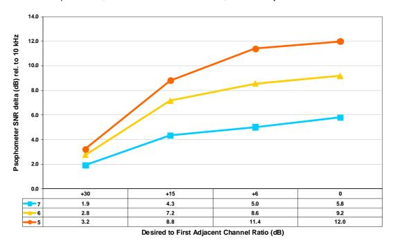
Figure 8. Effect of transmission bandwidth on received SNR
