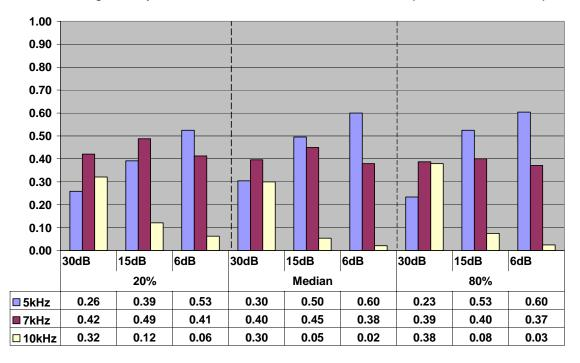
Figure 4: Speech Results for Three Receiver Bandwidths (20%, Median, and 80%)
