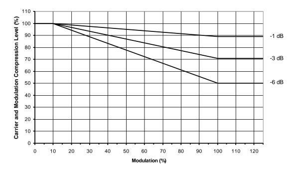
Figure 1. Amplitude Modulation Companding (AMC) compression function.
