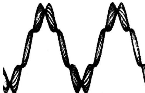
Figure 3. An example from the Inovonics 730 user manual of a properly synchronized RDS subcarrier in quadrature with the pilot, as shown from an oscilloscope
