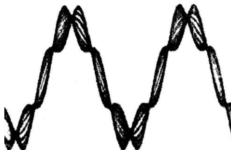
Figure 3. Oscilloscope view of a synchronized RDS subcarrier in quadrature with the pilot (Source: Inovonics 730 user manual)
