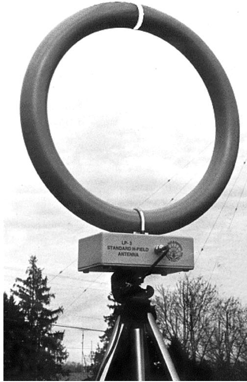
Figure 10. AM field measurements are best made with a good quality shielded loop antenna. (Courtesy of Chris Scott & Associates)
