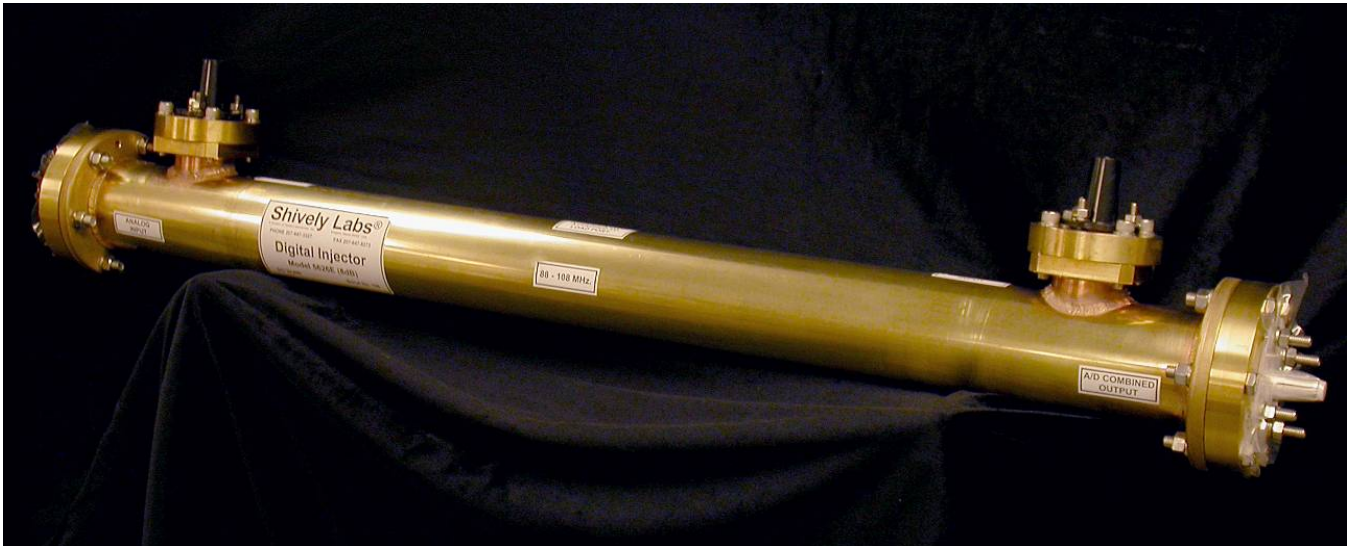
Figure 2. High-power combiners such as the one shown here are used to combine the outputs of separate analog and digital transmitters and require a dummy load which will typically dissipate a significant amount of power. (Courtesy of Shively Labs)
