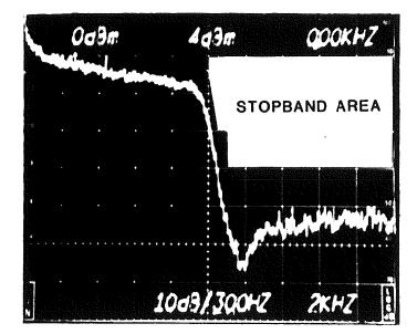
STOPBAND SPECIFICATION COMPLIANCE MEASUREMENT, USING PULSED-USASI NOISE SOURCE
