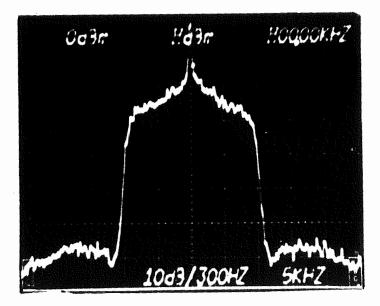
FIGURE 9 Same test as figure 2 except pulsed - USASI noise used in lieu of program audio.
