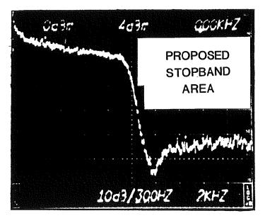
FIGURE 13 Stopband specification compliance measurement, using pulsed - USASI noise source.
