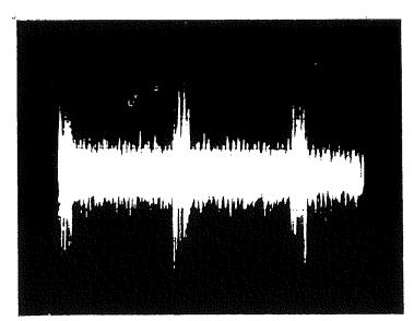
FIGURE 7 Pulsed - USASI Noise Test Signal
