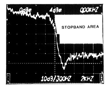
STOPBAND SPECIFICATION COMPLIANCE MEASUREMENT, USING PROGRAM AUDIO
