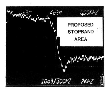
FIGURE 12 Stopband spcification compliance measurement, using program audio.
