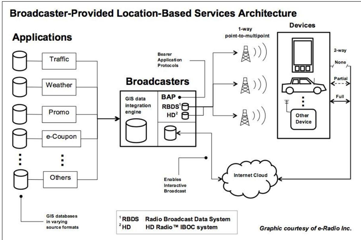
**Figure 1. LBS broadcast data architecture**
