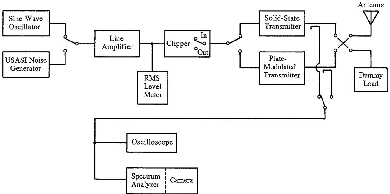
Figure 4. Transmitter Modulation Measurements - Equipment Configuration.
