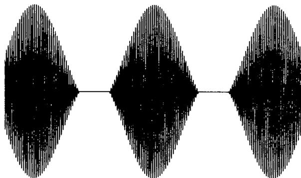
Figure 2. Overmodulation in a Typical AM Transmitter.
