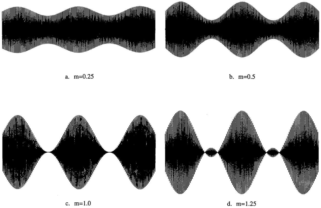
Figure 1. Waveforms of AM Carriers for Various Modulation Indices.
