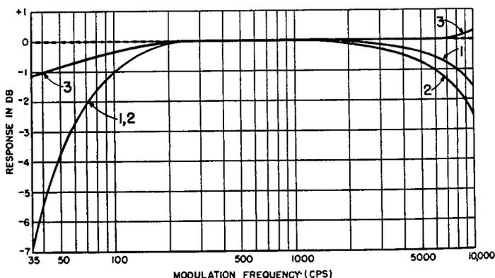
Fig. 5—Frequency characteristic curves for a 10-kw transmitter.
