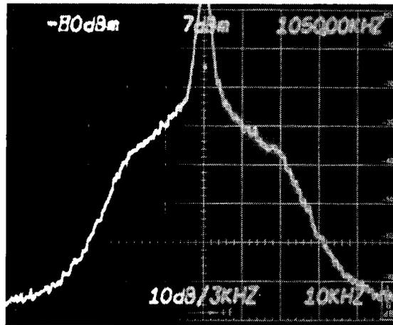
a. -3 dB input level (<100% peak modulation)
