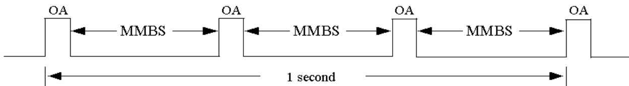
Figure P.3: Typical multiplex coding
