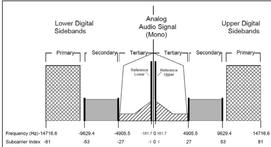
*Figure 10. Hybrid AM IBOC spectrum – 5 kHz analog signal bandwidth<sup>8</sup>*
