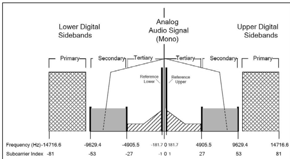
*Figure 11. Hybrid AM IBOC spectrum – 8 kHz analog signal bandwidth<sup>9</sup>*
