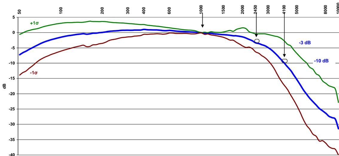
Figure 18 illustrates the combined frequency response of all receivers through the test bed (blue line), with the -3 dB point at 2450 Hz and the -10 dB point at 4100 Hz. The overall variation in audio bandwidths is shown by the standard deviation for the entire test population in green ( $\sigma+1$ ) and brown ( $\sigma-1$ ). For example, first-order standard deviation at the -10 dB point is approximately -2.6 dB and -17.2 dB, a range of 14.6 dB.
