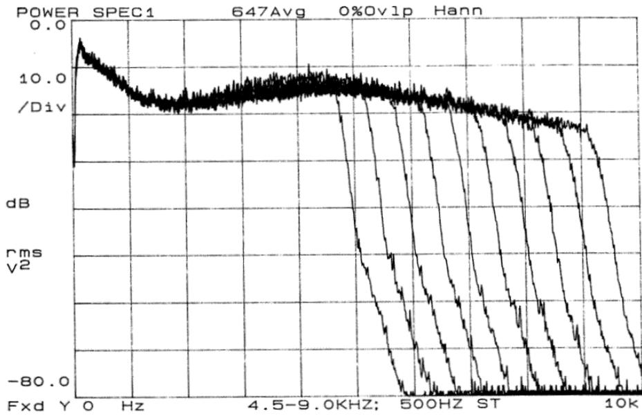
**Figure M-5 - Spectral output mask of Omnia 5EX processor using USASI noise at lowpass filter bandwidths 10, 8, 7, 6, 5.5 and 5.**
