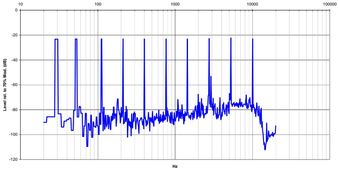
**Figure M-4 - Spectral output mask of Optimod 9200 using USASI noise at lowpass filter bandwidths from 4.5 kHz to 9.0 kHz in 500 Hz increments.**
