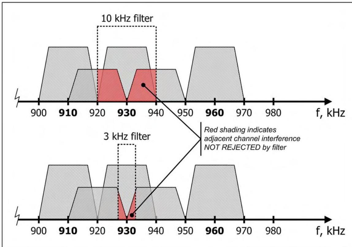
Figure 6. Illustration of the rejection of adjacent channel interference as a function of receiver filter bandwidth.
