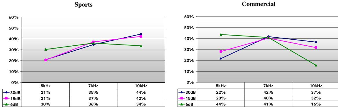
Figure 9. Percentages of listeners who picked one bandwidth over another, by genre, with no 1st-adjacent channel interference (30 dB), moderate 1st-adjacent channel interference (15 dB), and heavy 1st-adjacent channel interference (6 dB)
