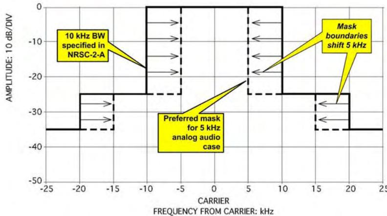
Figure 13. Illustration of preferred reduction of RF mask for example in Section 4.3
