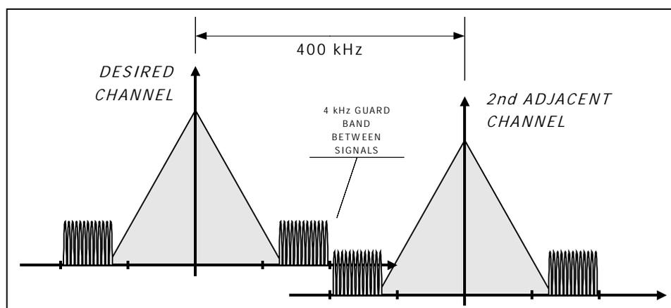
**Figure 3. Illustration of potential interference between 2nd-adjacent FM IBOC signals**
