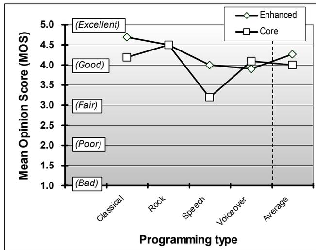
Figure 10. Comparison of AM IBOC subjective evaluation results for enhanced digital and core digital audio quality under laboratory AWGN conditions
