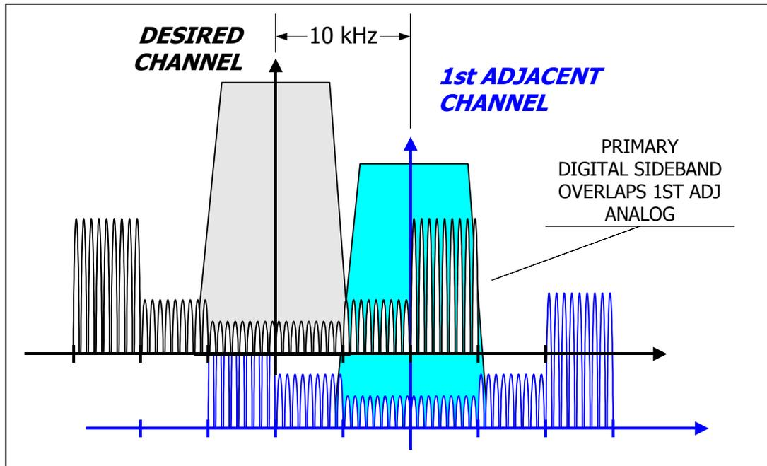
**Figure 2. Illustration of potential interference to/from 1<sup>st</sup>-adjacent analog signals by AM IBOC digital sidebands**
