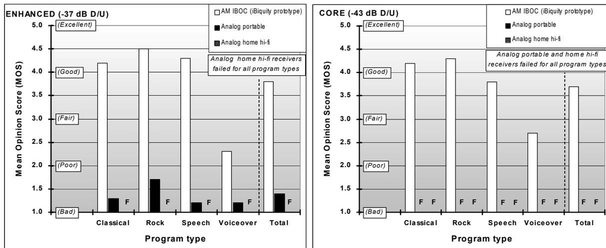
Figure 19. Comparison of AM IBOC and analog audio subjective evaluation results obtained in the laboratory with single 3<sup>rd</sup>-adjacent channel interference
