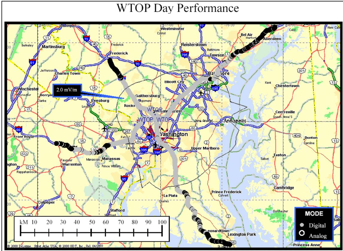
Figure 24. Coverage map including IBOC digital coverage (on radials) and 2 mV/m contour
