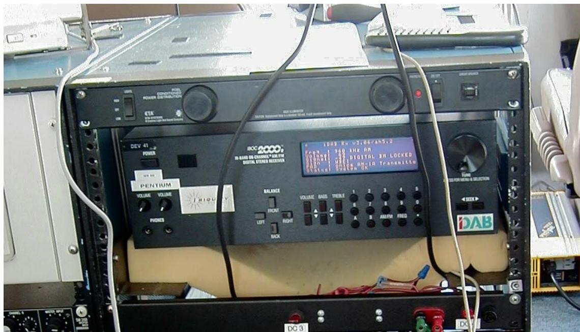
Figure 7. iBiquity prototype receiver –as used in field test vehicle
