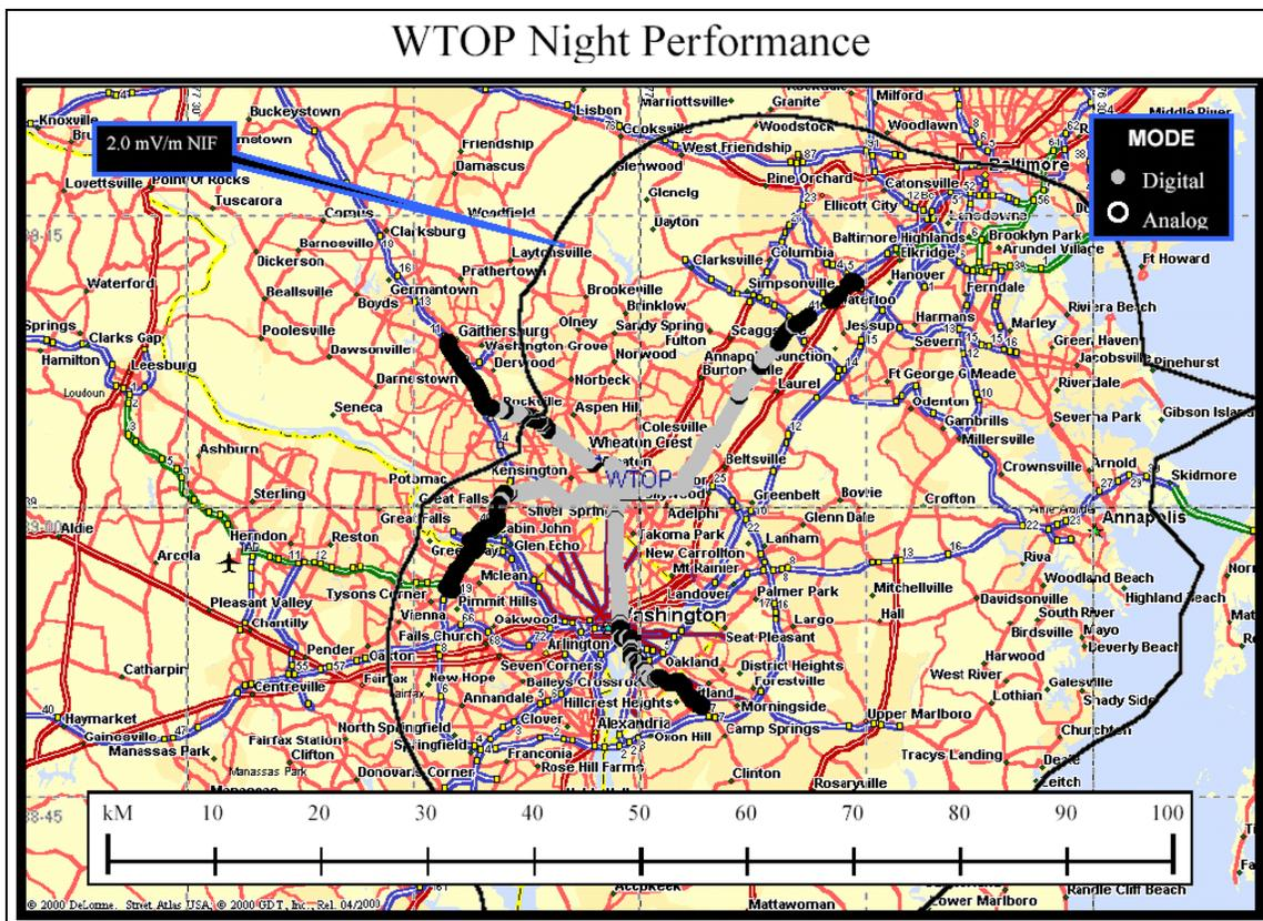
**Figure 25. Coverage map including IBOC digital coverage (on radials) and NIF contour**
