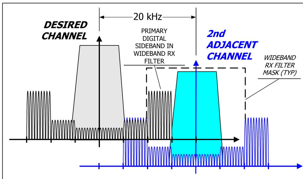
Figure 3. Illustration of potential interference between 2<sup>nd</sup>-adjacent AM IBOC signals
