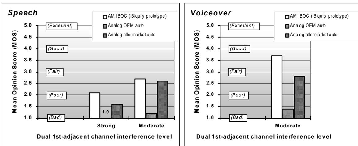
**Figure 15. Comparison of AM IBOC and analog audio subjective evaluation field results with strong (0 to +3 dB D/U) and moderate (+8 to +15 dB D/U) dual 1<sup>st</sup>-adjacent channel interference**
