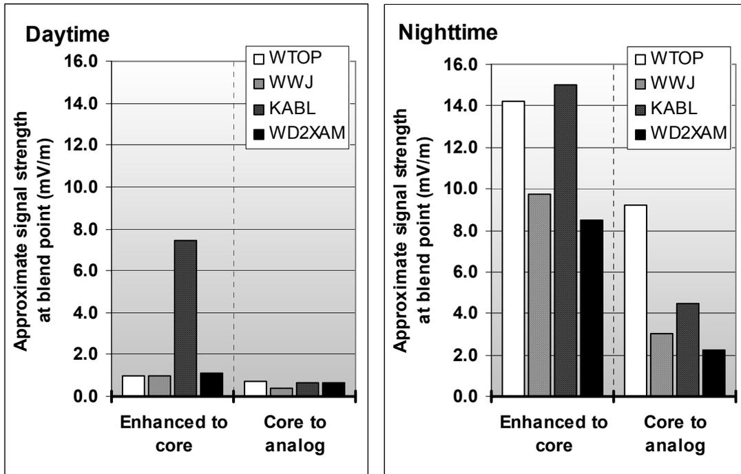
**Figure 23. Approximate signal strength at blend points for field test stations (for each station, results averaged over all test radials)**
