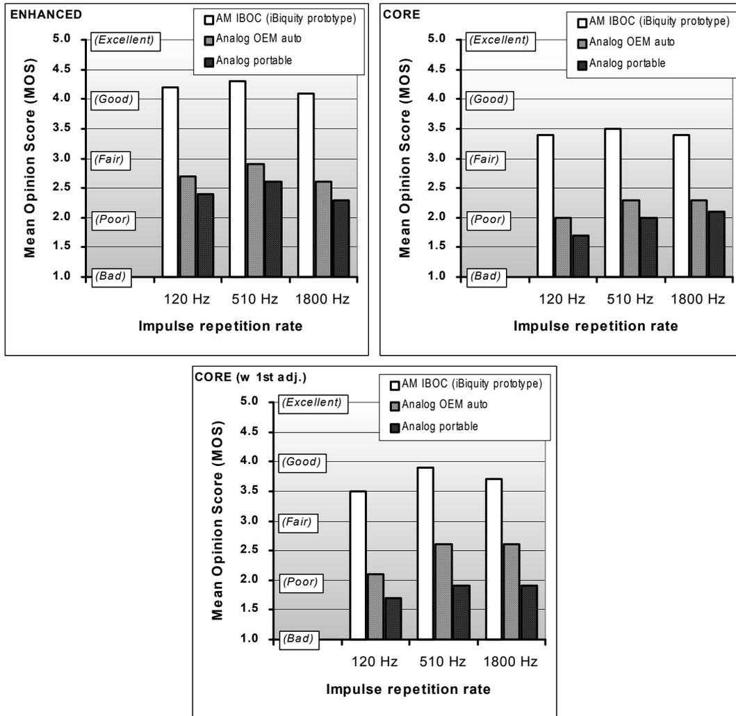
**Figure 12. Comparison of AM IBOC and analog audio subjective evaluation results under laboratory impulse noise conditions (aggregated for all program types)**
