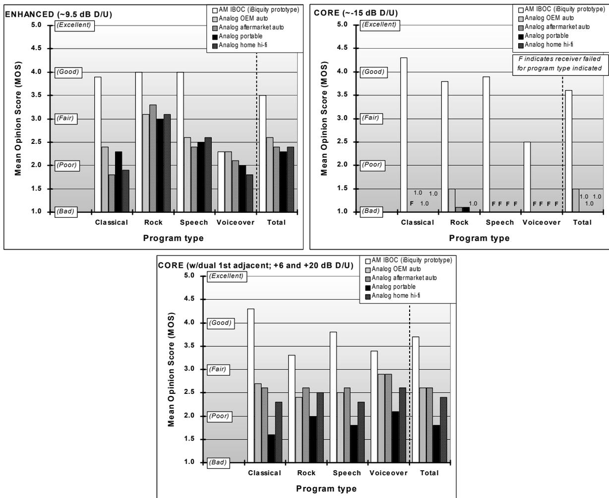
Figure 14. Comparison of AM IBOC and analog audio subjective evaluation results obtained in the laboratory with 1<sup>st</sup>-adjacent channel interference
