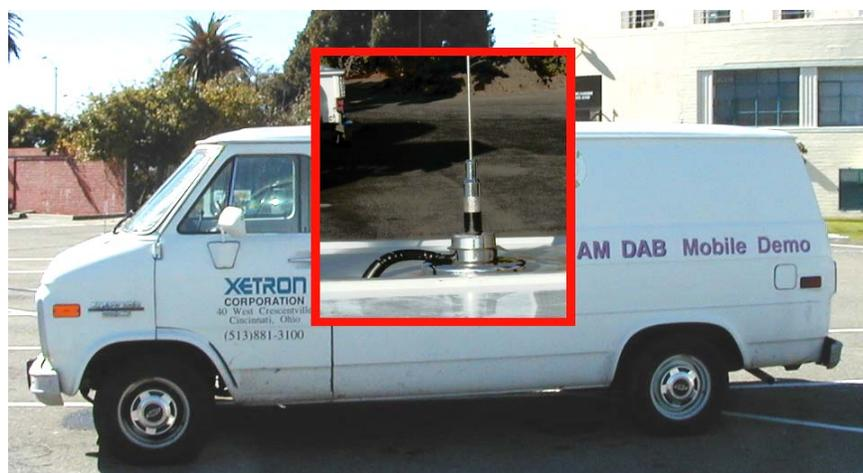
Figure 5. Field test vehicle and roof-mounted receive antenna (inset)
