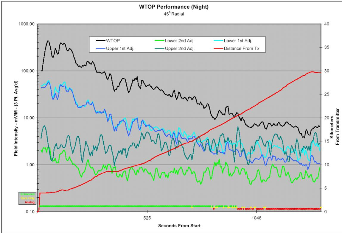
**Figure 22. Field test signal strength graph, nighttime (WTOP, 45° radial)**
