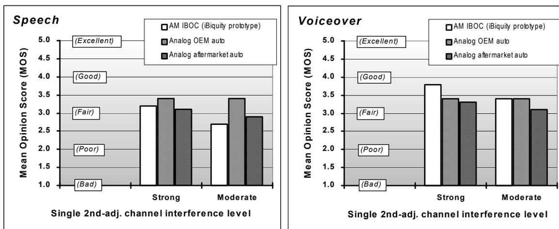
Figure 18. Comparison of AM IBOC and analog audio subjective evaluation field results with strong (-7 to -12 dB D/U) and moderate (+1 to -4 dB D/U) single 2<sup>nd</sup>-adjacent channel interference
