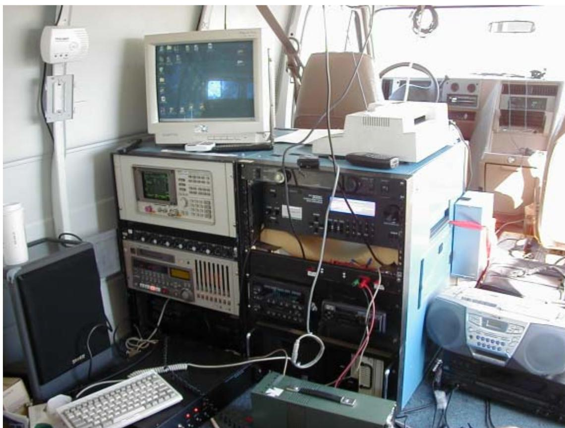
Figure 6. Interior view of field test vehicle showing analog and IBOC receivers, computer, and test equipment
