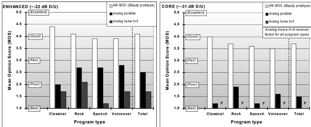
**Figure 16. Comparison of AM IBOC and analog audio subjective evaluation results obtained in the laboratory with single 2<sup>nd</sup>-adjacent channel interference**
