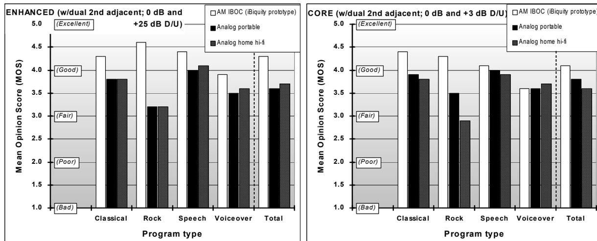
Figure 17. Comparison of AM IBOC and analog audio subjective evaluation results obtained in the laboratory with dual 2<sup>nd</sup>-adjacent channel interference
