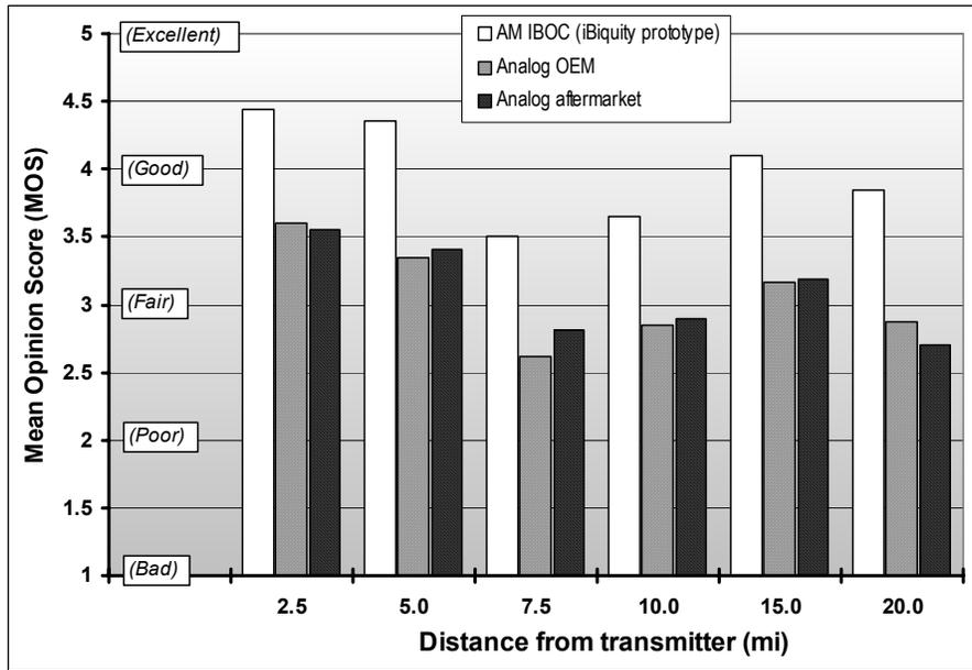
Figure 9. Comparison of AM IBOC and analog subjective evaluation results for WD2XAM<sup>22</sup>
