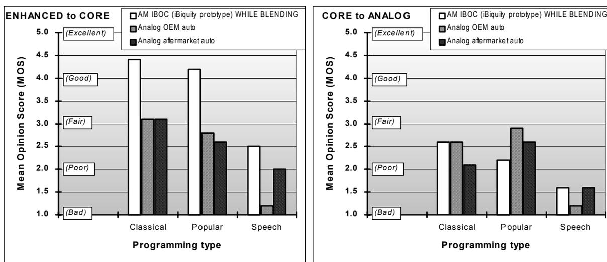
**Figure 26. Comparison of AM IBOC and analog audio subjective evaluation field results at “blend to analog” operating point**
