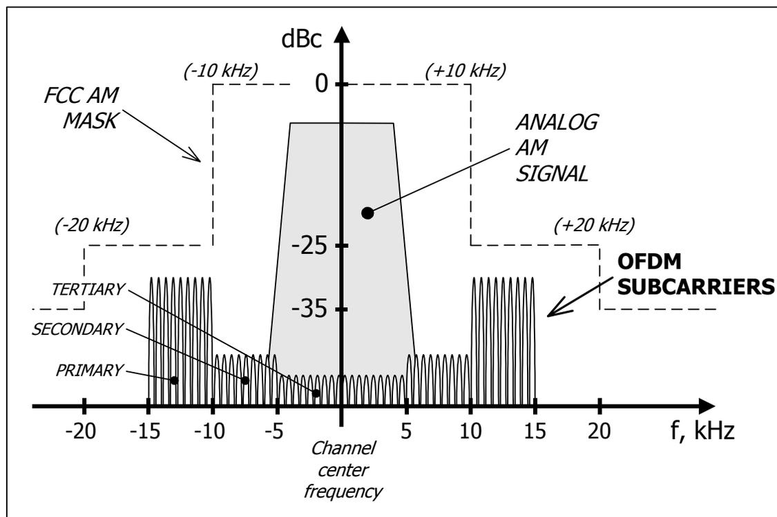
**Figure 1. iBiquity AM IBOC system signal spectral power density**
