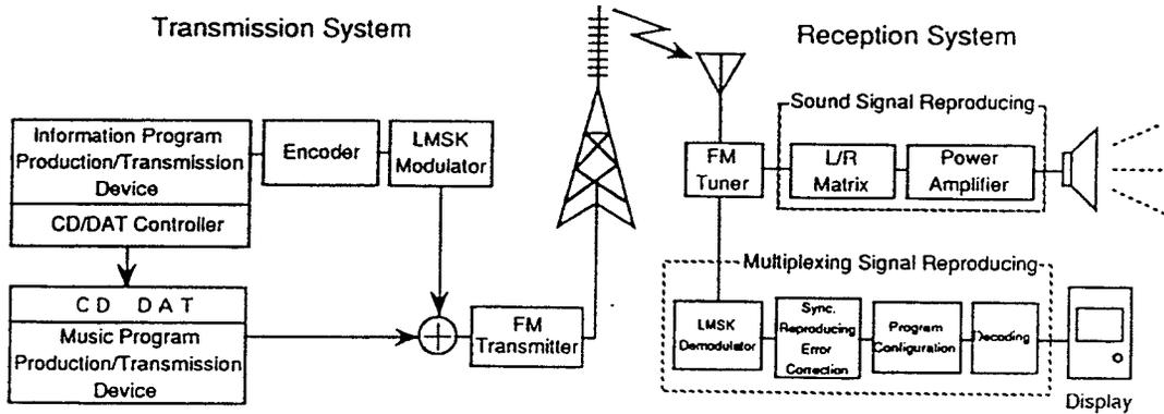
Figure 2. FM multiplex broadcasting system
