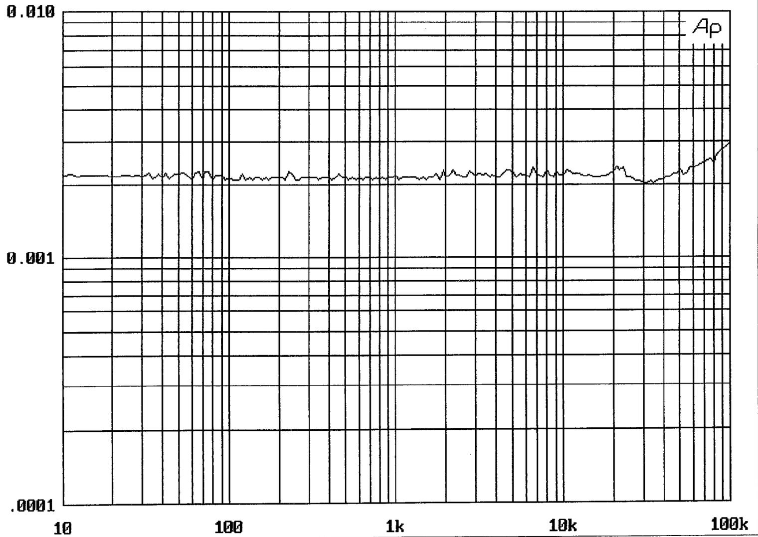
Bessel Null Fmod=31.188kHz: Dev=75kHz: 2-13-97
