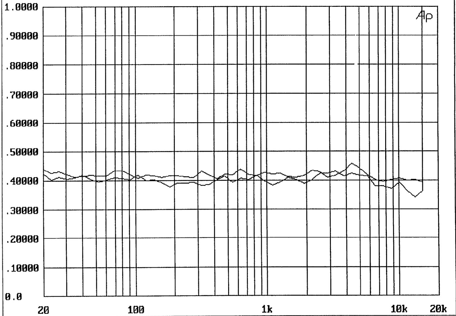
Digital DJ Separation L->R AMPL(dBr) & AMPL(dBr) vs FREQ(Hz) 23 DEC 96 10:50:45
