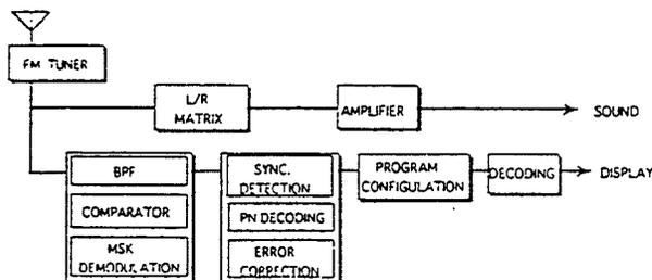
Figure 4. Block diagram of receiver
