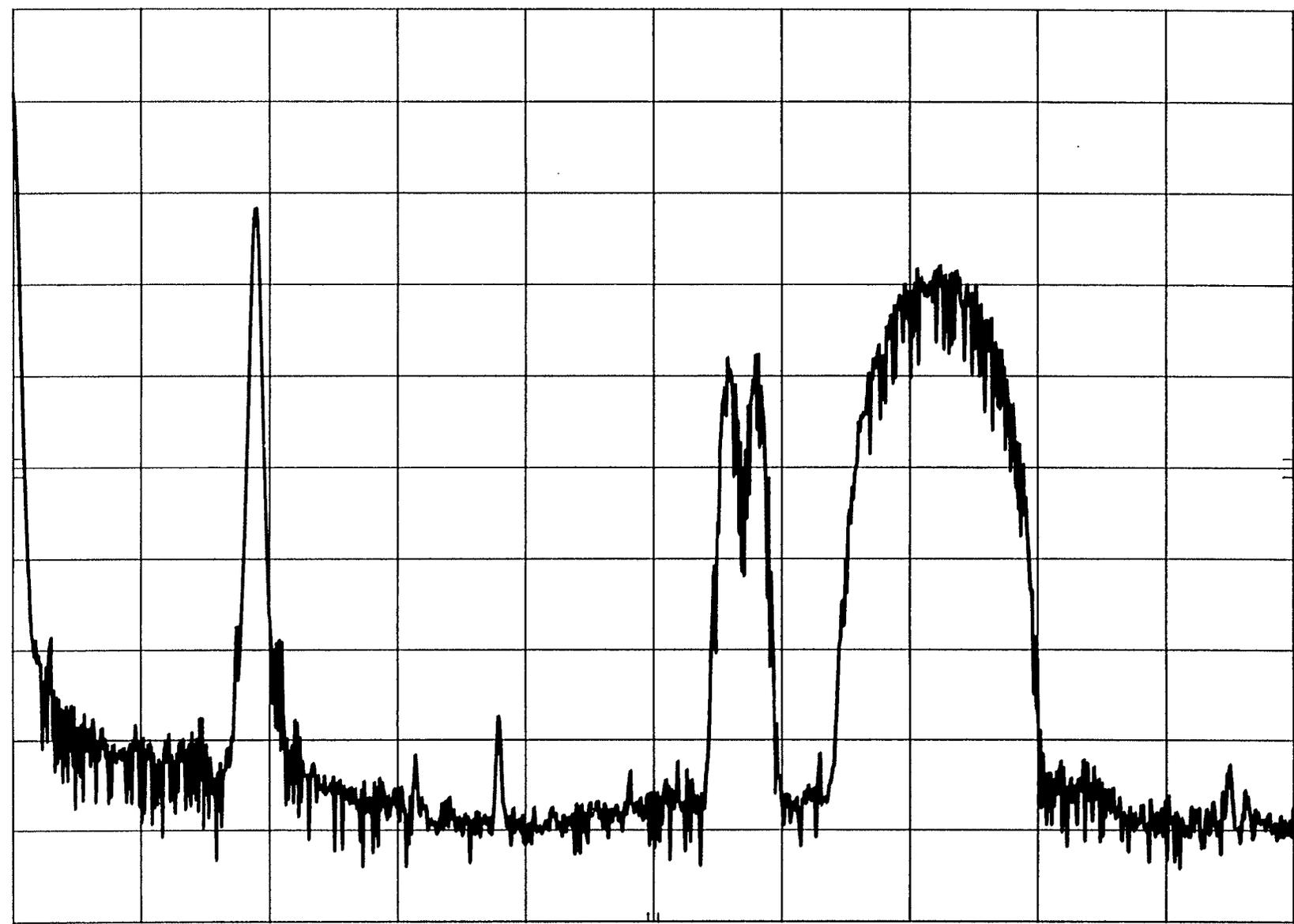
START 0 Hz RES BW 300 Hz VBW 30 Hz STOP 100 kHz SWP 30.0 sec
