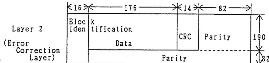
Figure 5. Frame structure of product code (279,190)\*(279,190)
