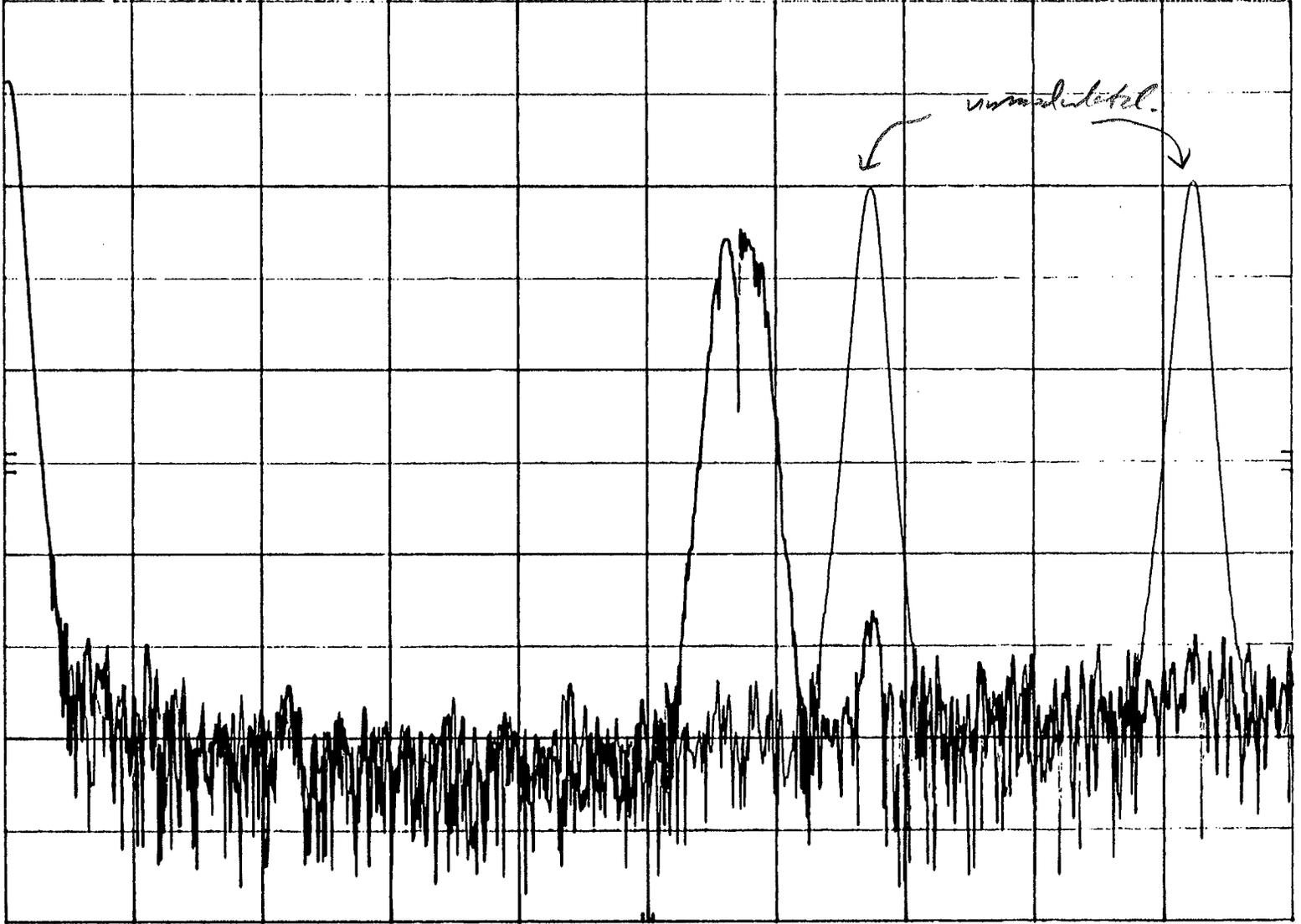
START 0 Hz RES BW 1 kHz VBW 3 kHz STOP 100 kHz SWP 300 msec
