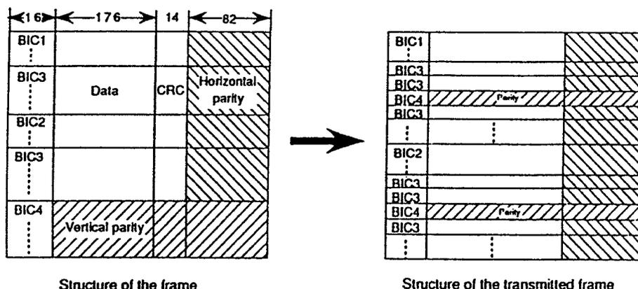
Figure 3. Structure of the frame
