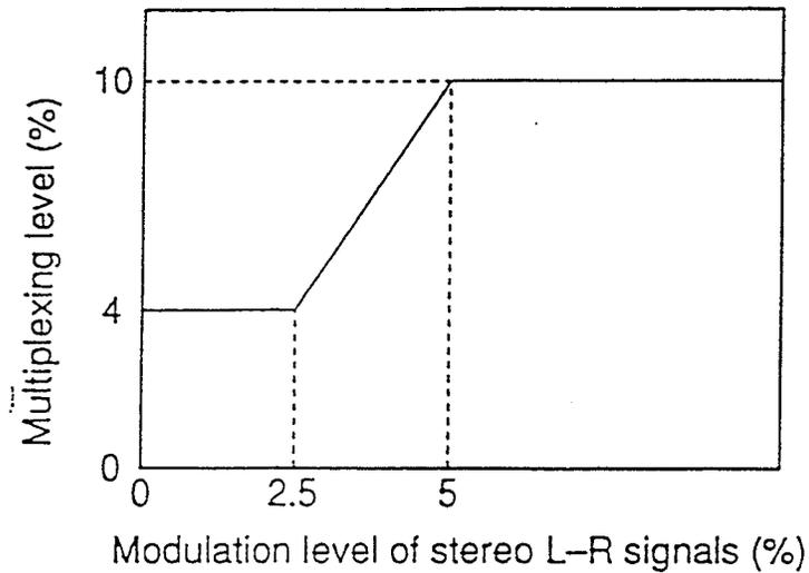
Figure 3. L-MSK method level control characteristics.
