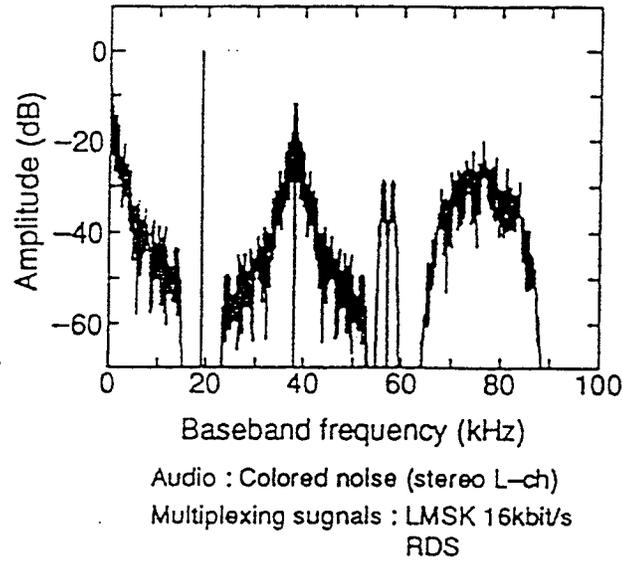
Figure 2. Baseband spectrum of L-MSK signal with RDS signals
