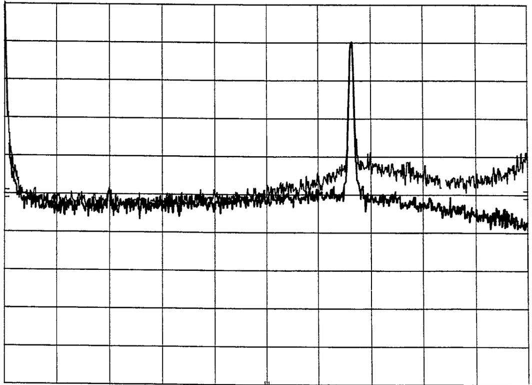
CENTER 50 kHz RES BW 300 Hz VBW 1 kHz SPAN 100 kHz
