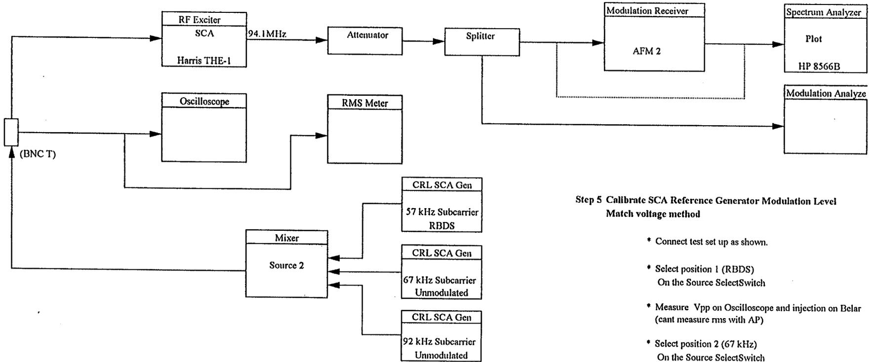
**Step 5 Calibrate SCA Reference Generator Modulation Level
