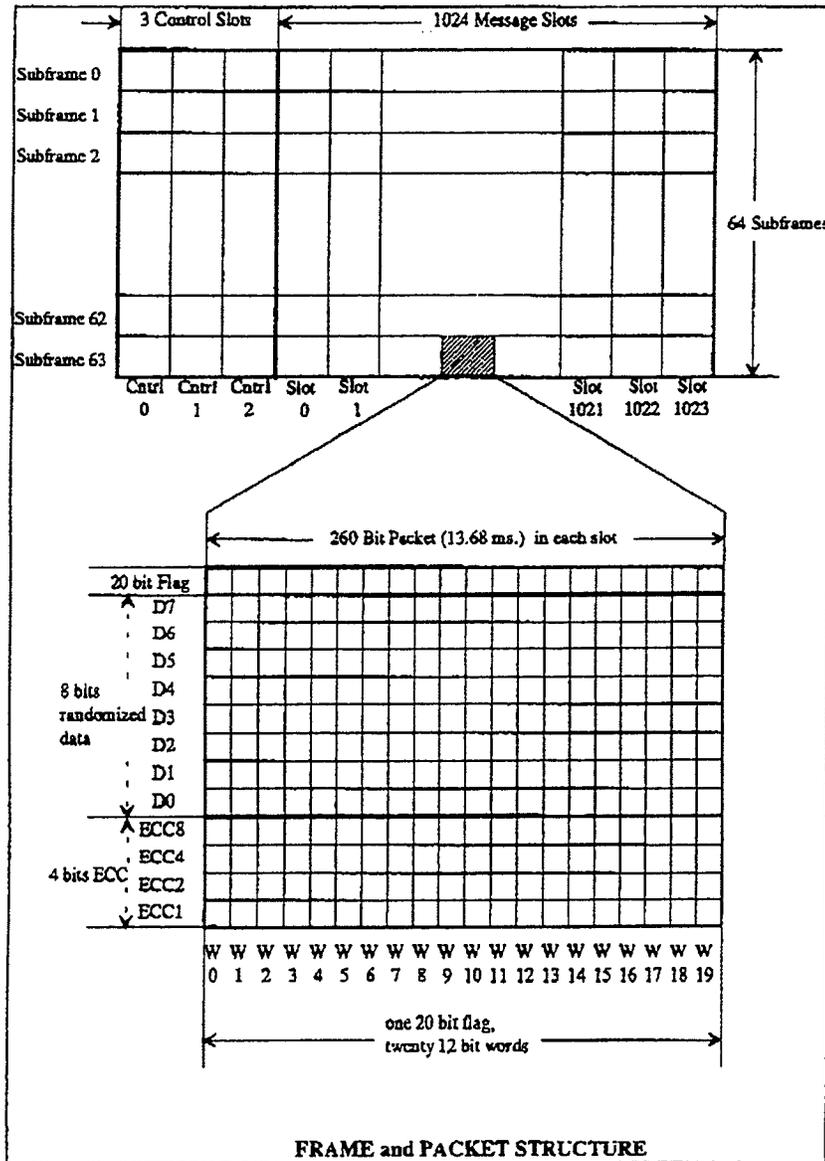
Figure 2 Frame and Packet Structure
