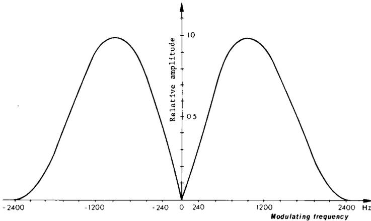
Figure 5: Spectrum of biphase coded radio-data signals
