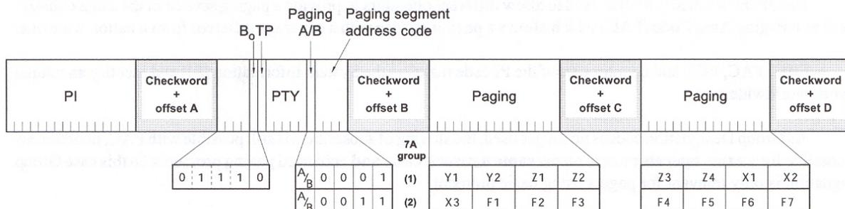
The paging segment address code is used to indicate the contents of block 3 and 4 in respective groups:
