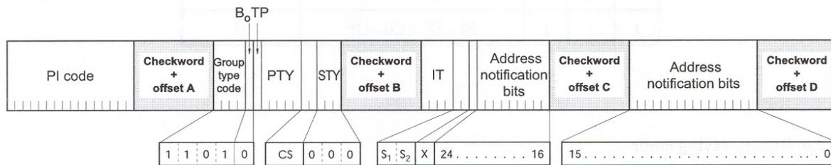
Figure M.11a: sub type 000 - Group type 13A
