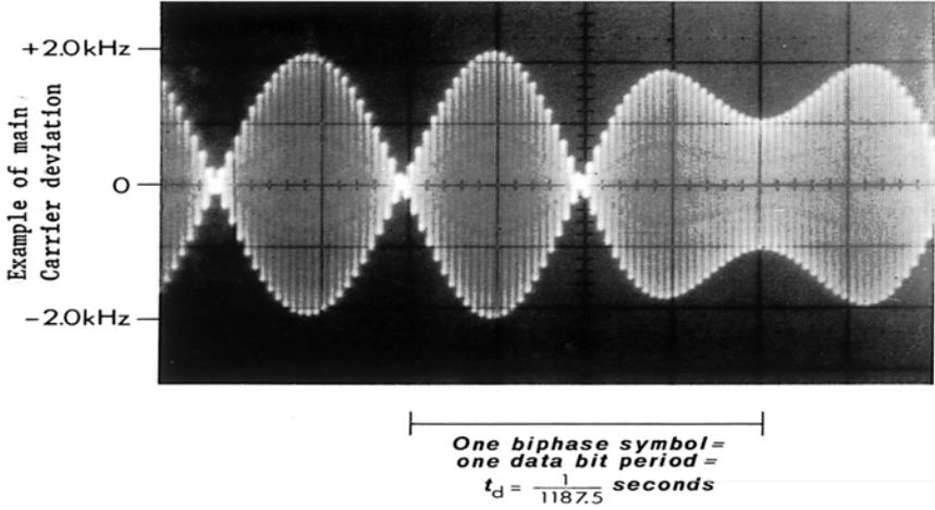
Figure 7: 57 kHz radio-data signals
