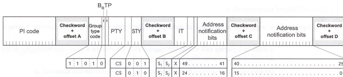
The 13A group, sub type 001, is used when 50 address notification bits (two 13A groups) are used. This group is immediately located after the 1A group starting the interval and represent high order notification bits.
