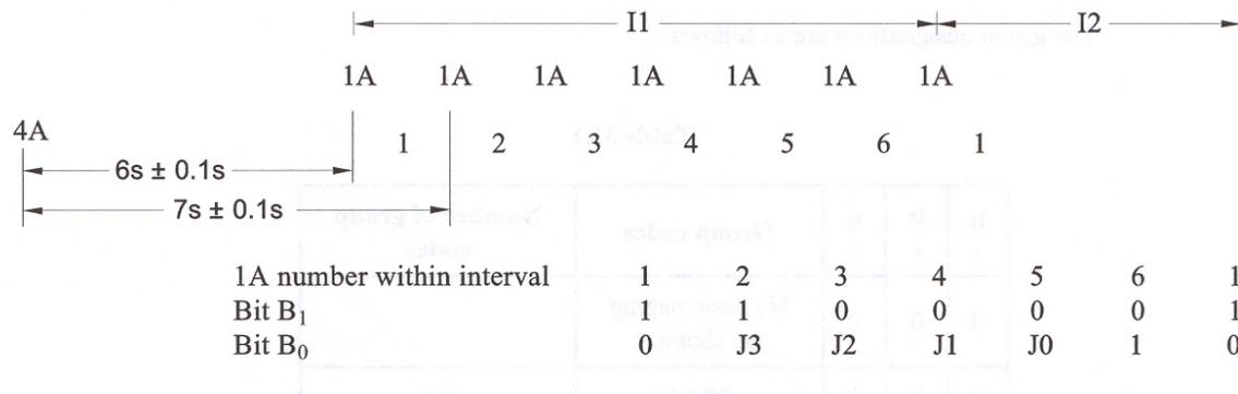
For battery saving purposes, each minute is divided into ten intervals of equal length (I0 ... I9). Each paging receiver belongs to the interval corresponding to the last digit of its individual code (digit 0 belongs to I0 and so on). Paging calls are placed within the interval corresponding to the last digit or within the two intervals following that interval.
