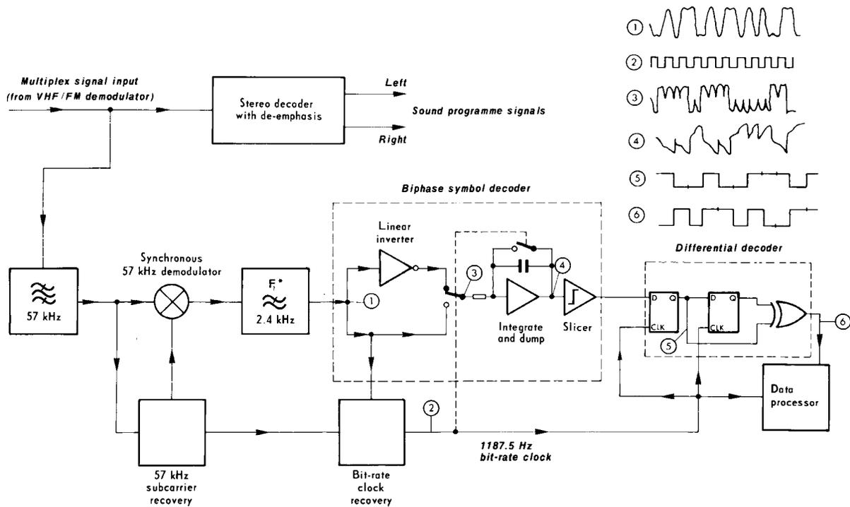
Figure 2: Block diagram of a typical radio-data receiver/decoder
