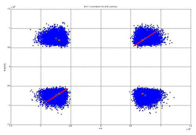
Figure B-2: IBOC Constellation with PAPR Reduction Enabled - No Added Noise
