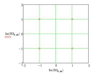
Figure A-5: Demodulated OFDM Symbol Constellation
