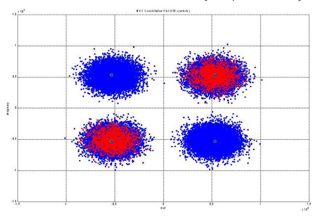
Figure B-9: IBOC Constellation with PAPR Reduction Disabled – Cd/No = 64 dB-Hz
