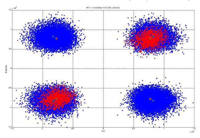
Figure B-3: IBOC Constellation with PAPR Reduction Enabled – Cd/No = 68 dB-Hz
