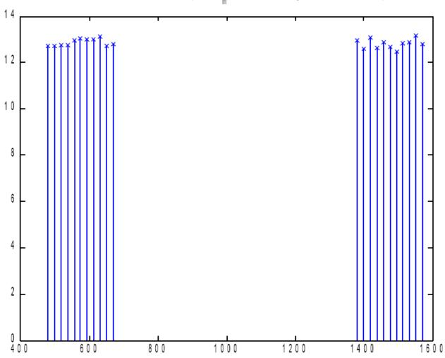
Figure B-19: Reference MER with PAPR Reduction Disabled - Cd/No = 64 dB-Hz
