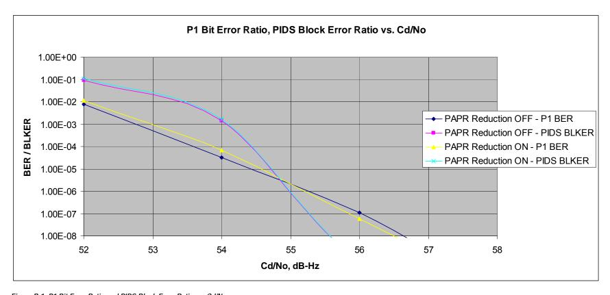
Figure B-1: P1 Bit Error Ratio and PIDS Block Error Ratio vs. Cd/No
