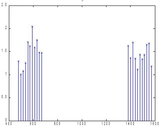
Figure B-21: Reference MER with PAPR Reduction Disabled – Cd/No = 52 dB-Hz
