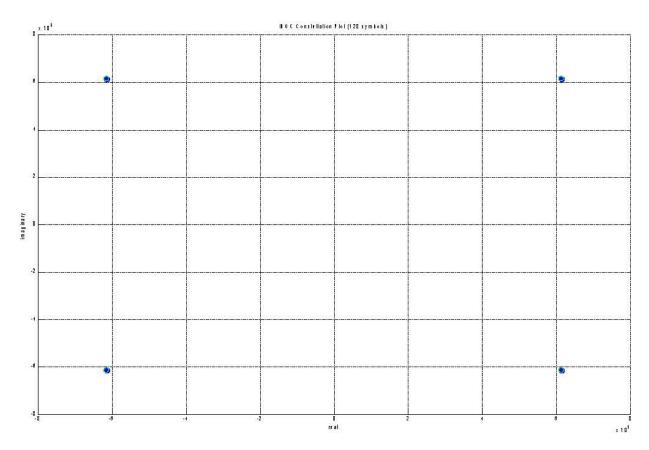
Figure B-7: IBOC Constellation with PAPR Reduction Disabled – No Added Noise
