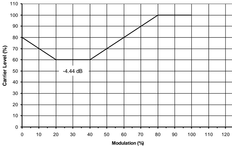
Figure 3. DCS example 2 – carrier compression function
