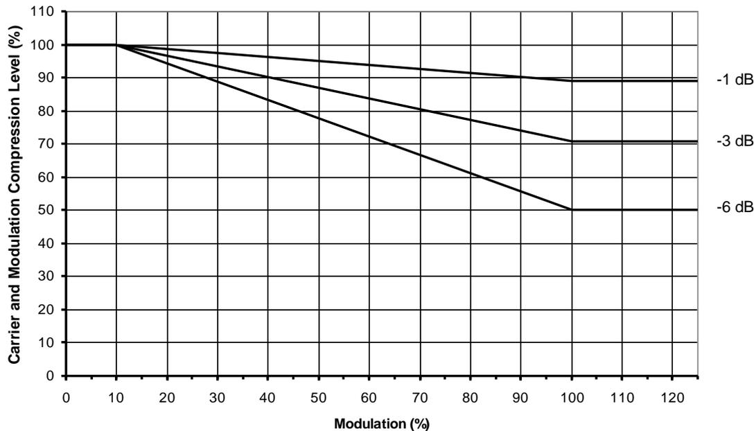
**Figure 1. Amplitude Modulation Comping (AMC) compression function.**
