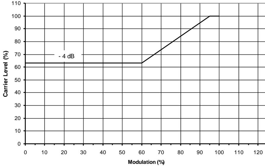
Figure 2. DCS example 1 – carrier compression function
