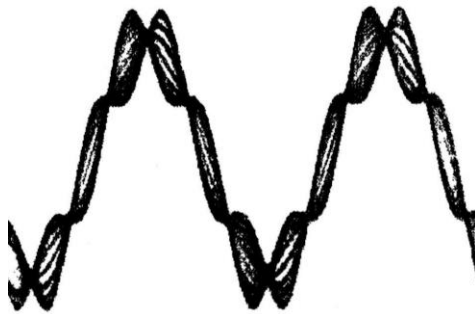
Figure 3. Oscilloscope view of a synchronized RDS subcarrier in quadrature with the pilot (Source: Inovonics 730 user manual)
