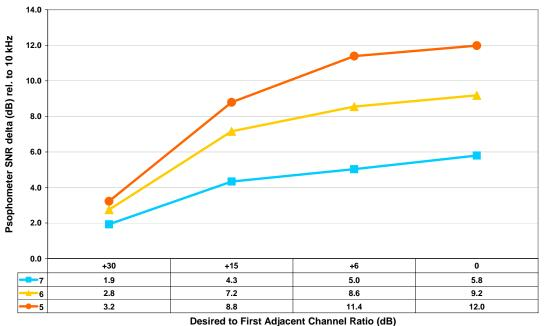
Desired to First Adjacent Channel Ratio (db)
