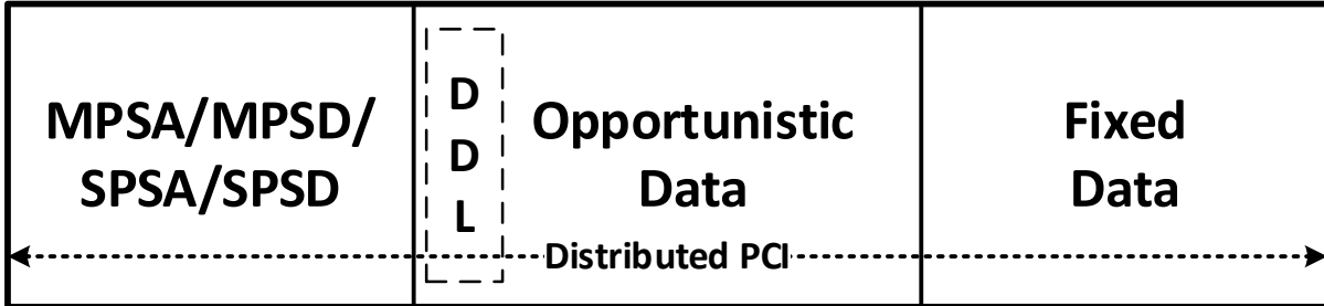
Figure 5-1: Standard L2 PDU Structure
